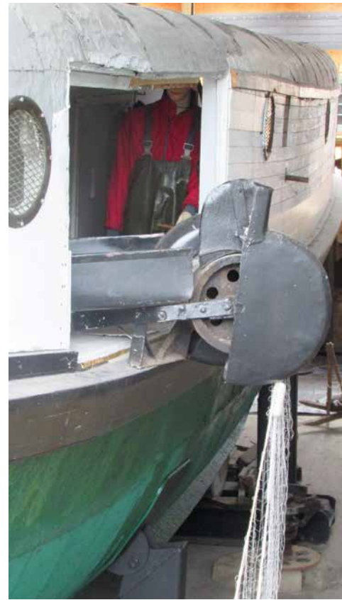
Net lifter from the fish tug Katherine V, Besser Museum, Alpena. Photo by S.A. McFerran.
