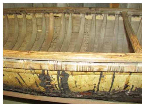
Mid-ships pirogue. Cedar ribs press thin cedar planks against birch bark. From the collection of Besser Museum, Alpena.
