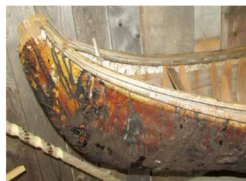
Birch pirogue. Spruce roots are dug and split. They are used to lash birch to gunwhales. From the collection of Besser Museum, Alpena.
