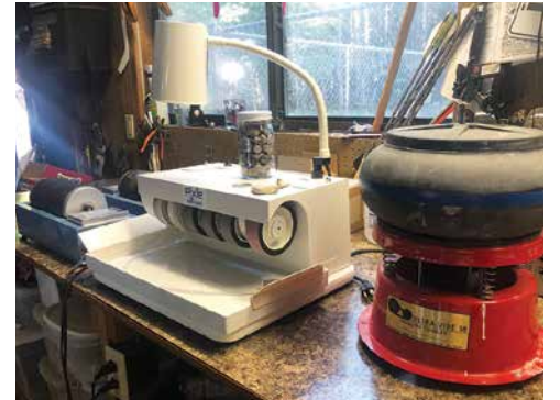
(L to R) Rock tumblers, Pixie lapidary machine and a vibrating tumbler.
