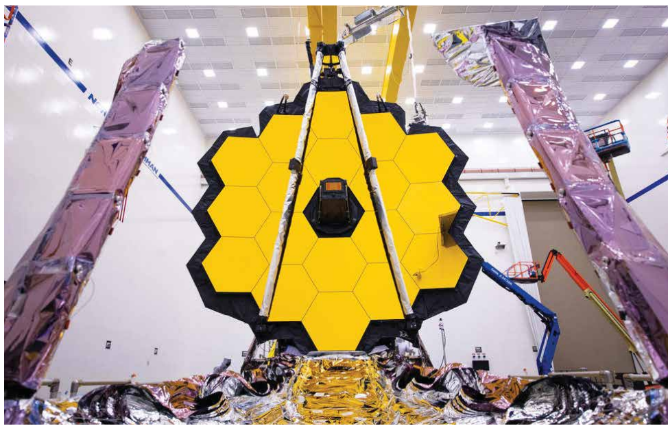
The James Webb Space Telescope, with fully deployed sunshield, in the assembly room. The sunshield will be folded up for launch. NASA photo.
