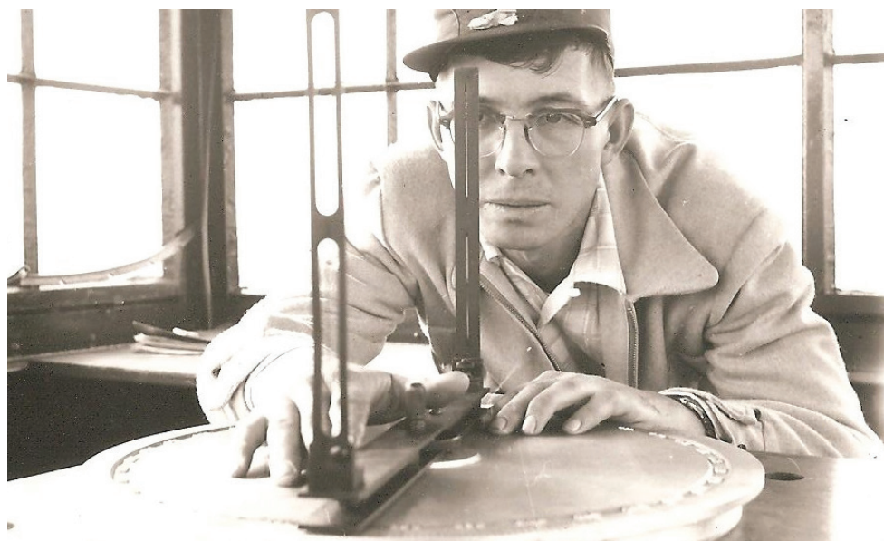
Wallace Humphrey using the Osborne Fire Finder device while manning the Glovers Lake Fire Tower, about 1950. Courtesy photo.
