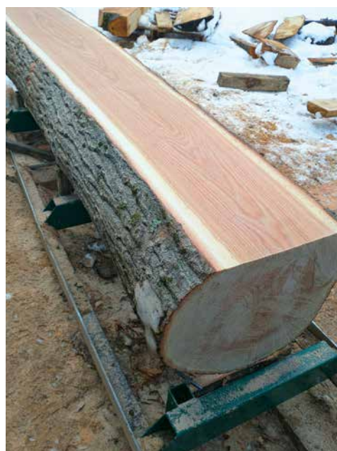
A log at the beginning of the milling process, after the first cut. The slab taken off the top of the log makes great firewood. Photo by Stewart A. McFerran.
