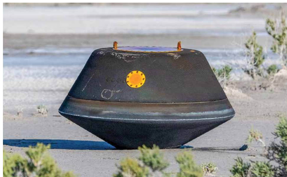
The sample capsule, post landing, in the Utah desert. The capsule's black color is from charring that occurred upon reentry. NASA courtesy photo.
